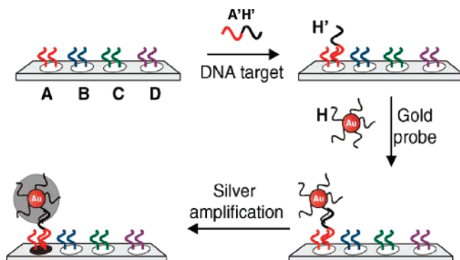
Figure 14. Schematic of DNA hybridization to microarrays and detection using Ag-amplified Au NP probes. Reprinted with permission from ref 346. Copyright Elsevier B.V.
